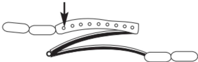
1. Depress the end of the spring bar on the centre clasp with a pin.
